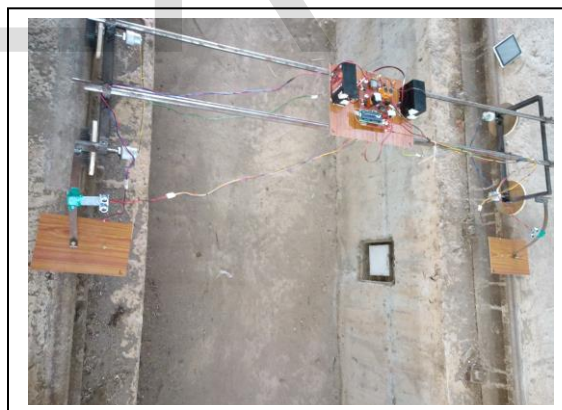
Figure 2. Technical railway crack detection system
